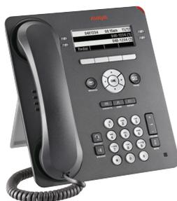
**9504 Model** – A cost-effective, digital phone with paperless labels and a four-line display with dual red/green LED buttons. Through the four interactive soft key buttons, users can “screen-scroll,” providing up to 12 programmable buttons.
