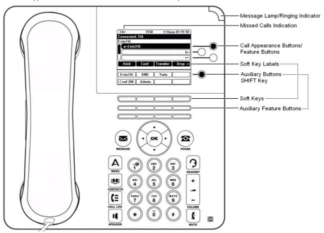
This phone supports 24 programmable call appearance/feature buttons. The labels for 3 of these buttons are visible on the main display and can be controlled by the adjacent buttons to the right. You can use the ▲ up and down ▼ arrow keys to scroll the display. You can also use the ◀ left and right ▶ arrow keys to move through the button features in pages of three.
