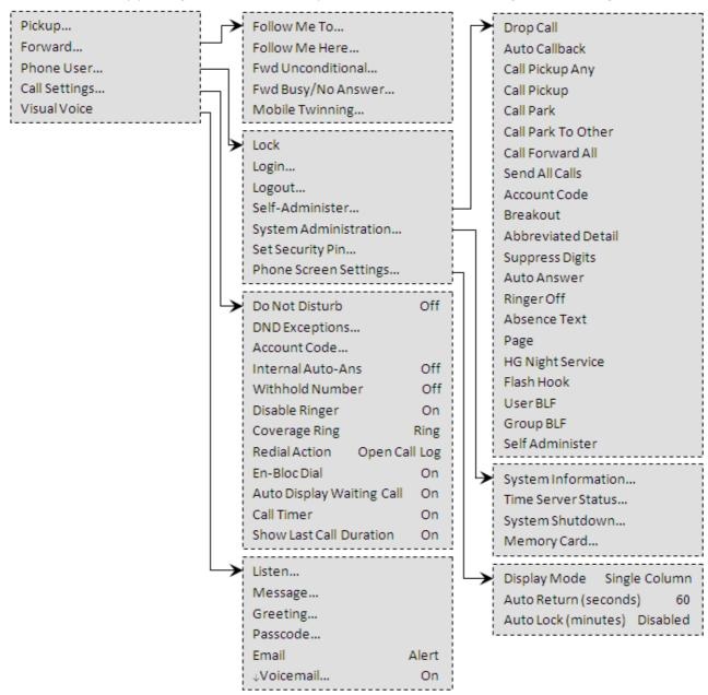
To exit the whole user menu and return to the appearance menu, press the **PHONE/EXIT** button or, if displayed, press the **Exit** soft key.
